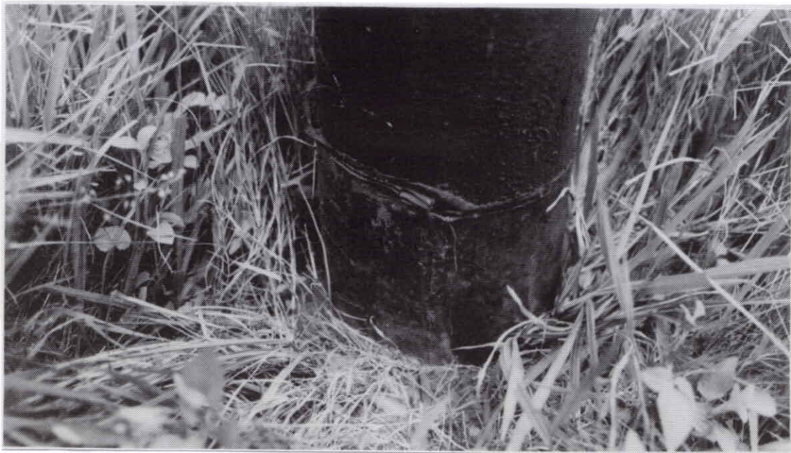
Fig. 2. Ground line of sub-standard transmission pole (treated with 80\text{kg.m}^{-3} creosote by the full cell process) after 12 months' service. No creosote was visible running down the sides of such poles, nor was the soil surrounding them polluted by creosote. In keeping with these observations, no bare soil existed and vegetation completely surrounded the poles.
